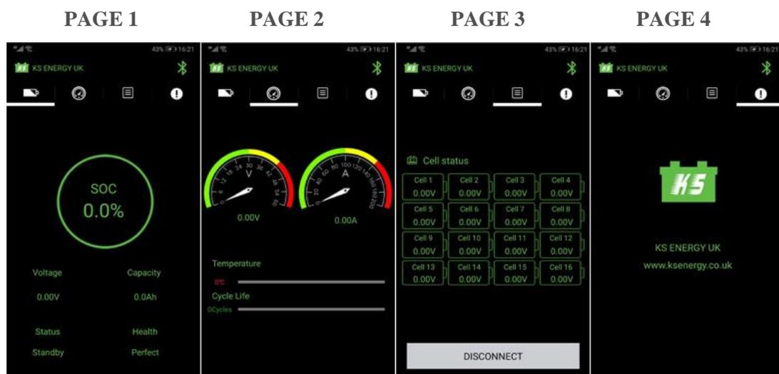
The battery information within the application is essentially self-explanatory and an overview follows: Page 1 displays State of Charge (SOC) as a percentage, the battery Voltage, total Capacity, and the present Status
